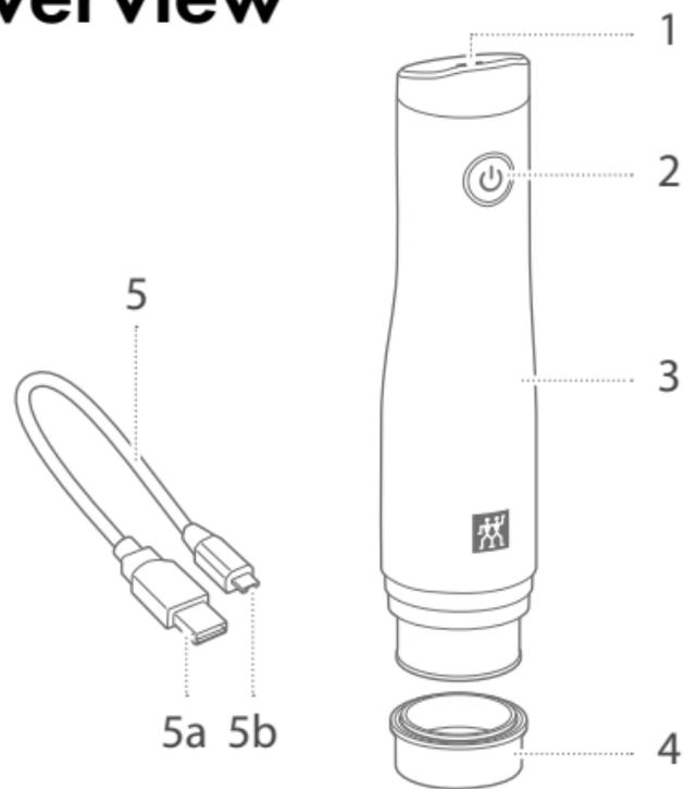
**1** Slot for the micro USB connector
